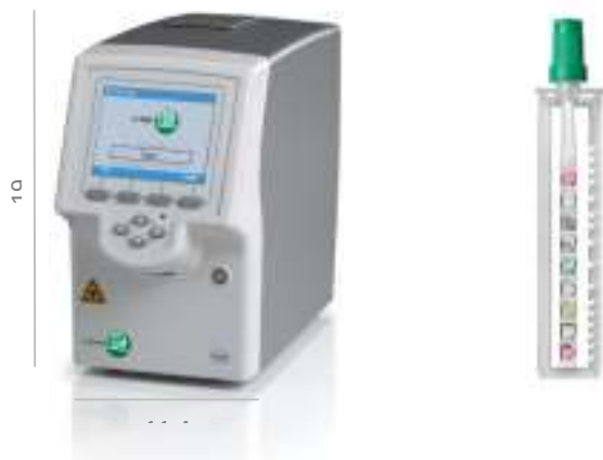
Figure 30. cobas® Liat® System. The cobas® Liat® Analyzer compresses the assay tube to move the sample and selectively release reagents from tube segments, under temperature-controlled conditions.
